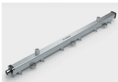
The hydrogen injection rail, equipped with pressure and temperature sensors, evenly directs gas to the injectors.
