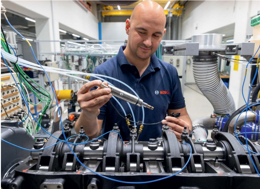
Tests with the new injector for direct hydrogen injection, first presented by Bosch at Agritechnica 2023 in Hanover, Germany.
