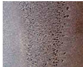
Insufficient coolant filtration can result in pitting. The result: damage to the cylinder due to corrosion.
