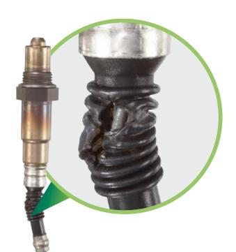
Lambda sensor condition: Damage on the molded cable tubing
