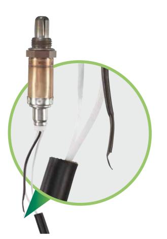
Lambda sensor condition: Broken cable
