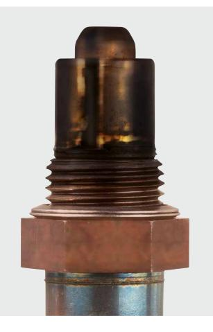
Lambda sensor condition: Black, with oily soiling
