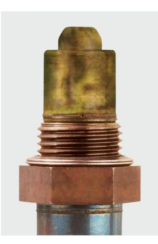
Lambda sensor condition: Green, grainy soiling
