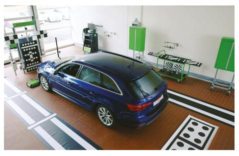
Calibration boards for camera systems, front radar and lidar systems, as well as calibration floor mats for rear and surround cameras and radar accessories for all kinds of radar systems are all available separately — so you can use these as building blocks to create a solution that suits your workshop.
