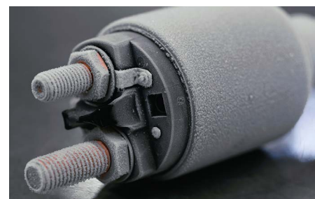
Cold storage, heat storage and changes in humidity to prove climate stability
