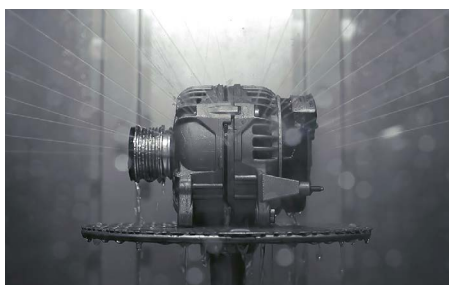
Splash water testing of tightness according to degrees of protection IPX4, IPX4K and IPX9K
