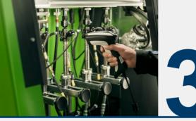
Labeling: The diesel component is labeled with a repair ID label or clip, and the QR code is subsequently scanned to enter the component data into the database on the QualityScan server
